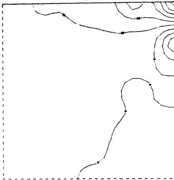
Figure 2. Expanded corner view of zero-Reynolds-number vorticity for a cavity.
